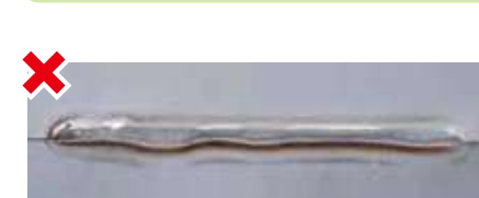
Meandered weld bead due to heat input shortage.
