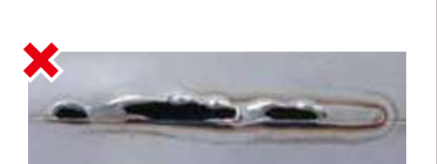
Burn-through caused by excessive heat input
